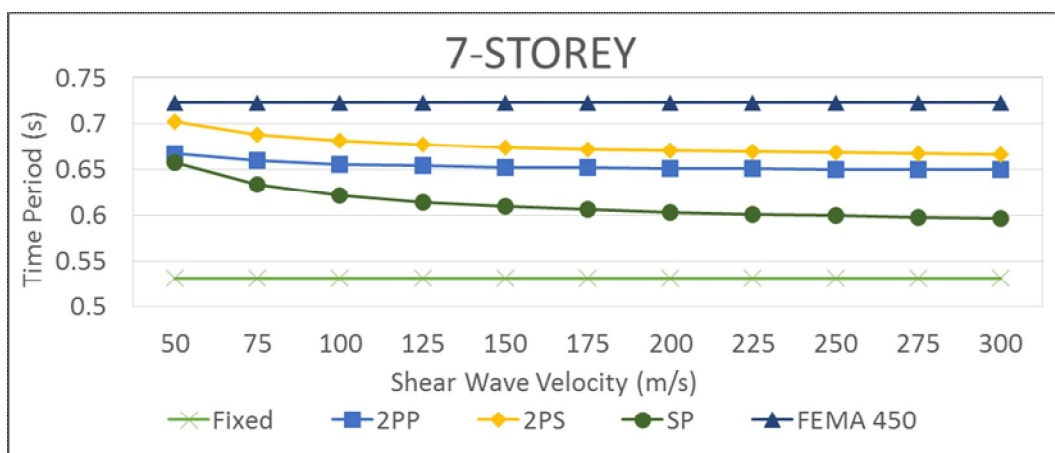
Fig. 4 Variation of T with Shear Wave Velocity (m/s) for 7-Storeyed Structure
